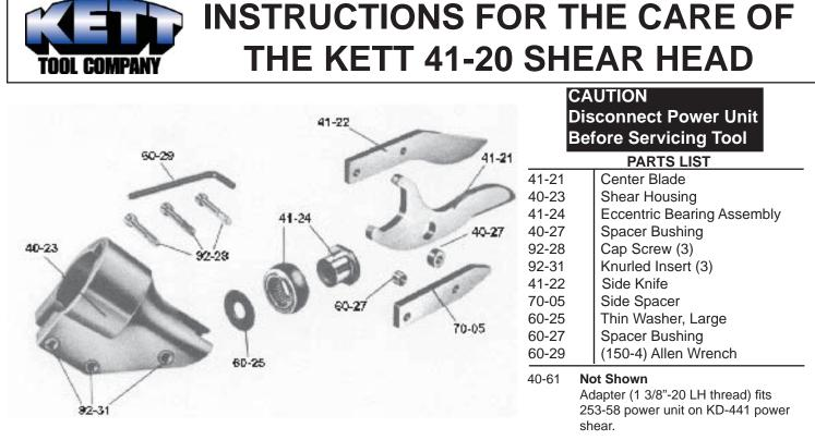
**DISASSEMBLY:** To remove the shear head from the motor loosen three cap screws (92-28). Remove shear head from motor by pulling head firmly forward. Slight tapping with a mallet may be required if head does not slide off easily.
